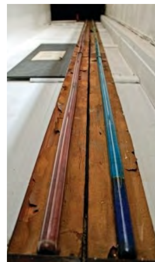
Lord Kelvin's diffusion experiment has been running a University of Glasgow lecture hall since 1872. Source: http://cen.acs.org/articles/91/i33/Old-Experiment-Even-Older-Curiosities.html
